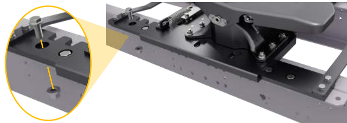
Mounting bolts used in the installation of the slider
