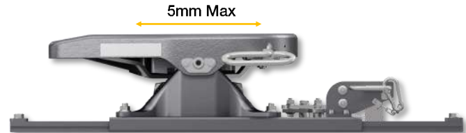
Limits of forward and rearward movement between carriage and rails
